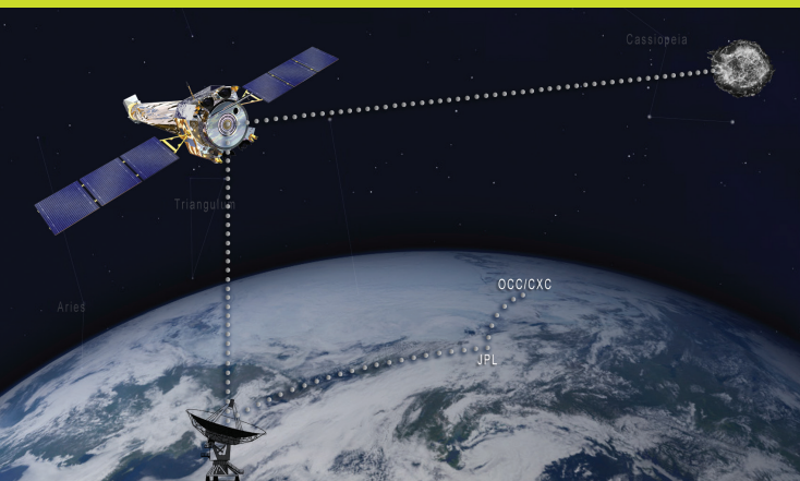
The data path from the cosmic source, to the satellite, to Earth. The data transmitted in binary code before being translated into a visual representation of the object. Credit: NASA/CXC/SAO
